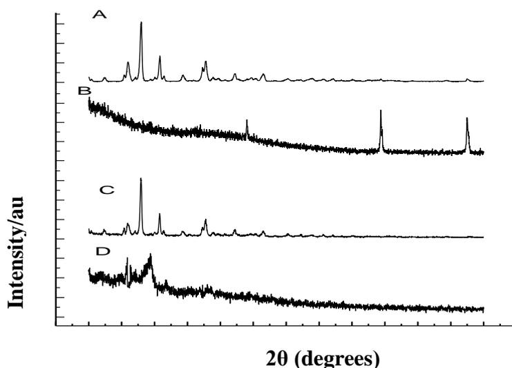
**Fig.1** X-ray diffractogram: ( A) MO, (B ) GA, (C) physical mixture,(D) MOGANPs
