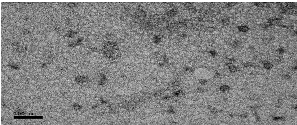
**Fig 2.** Transmission electron microscopy of MOGANPs nanoparticles
